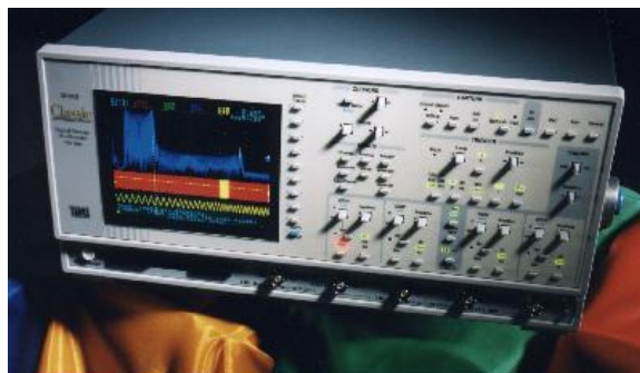
Figure 3.2.23: The Gould Classic 9500 Digital Storage Oscilloscope used in the experiments.
