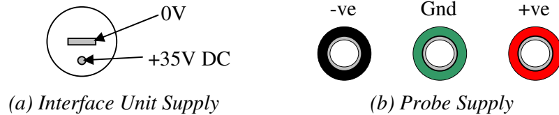
Figure 2.3.21: The power supply connections to the interface unit.
