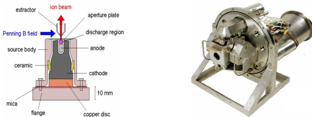
FIGURE 3 – Penning type source: (a) sketch; (b) source used in ISIS
