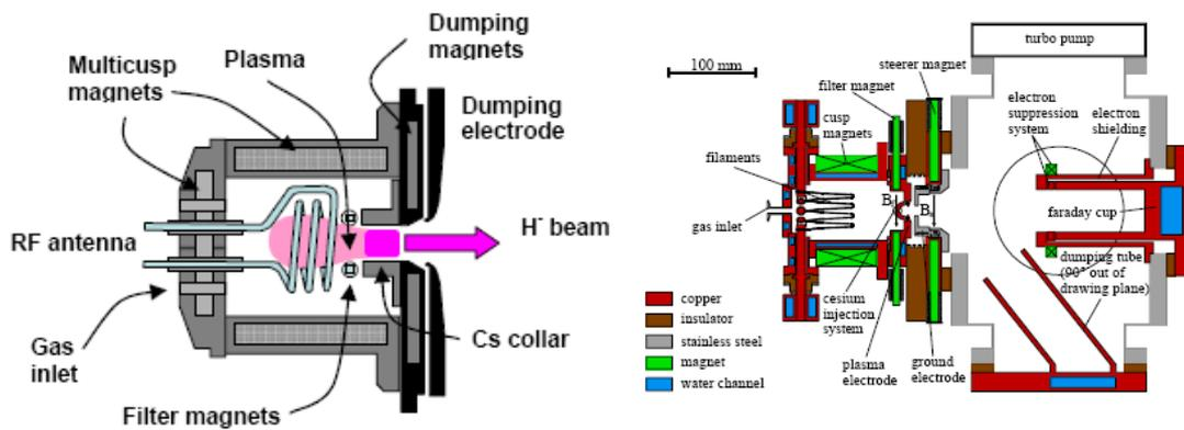
FIGURE 4 – (a) SNS (LBNL) source; (b) Source design for the ESS (IAP-Frankfurt)
