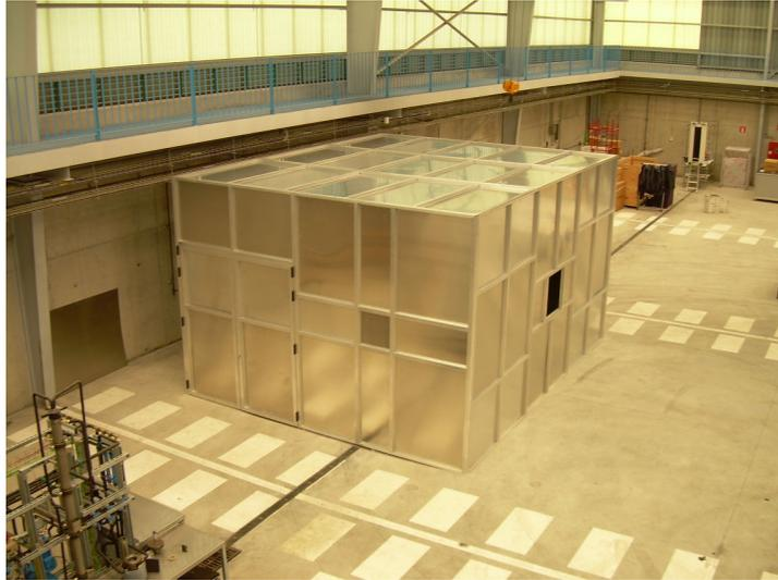
**FIGURE 1.** Faraday Cage of the ITUR ion source test stand at the Univ. Basque Country.
