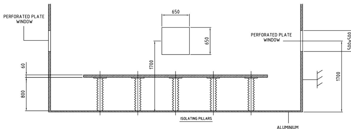
FIGURE 2. Sketch of the HV platform on 800 mm insulators
