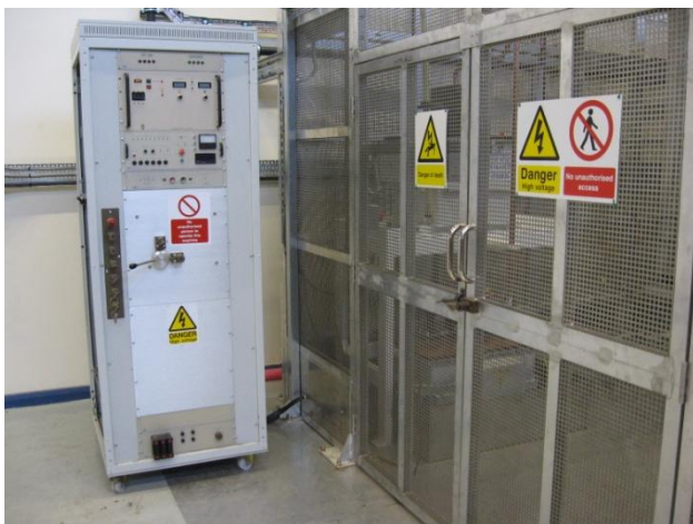
Figure 4: The platform bias DC power supply and the high voltage cage.
