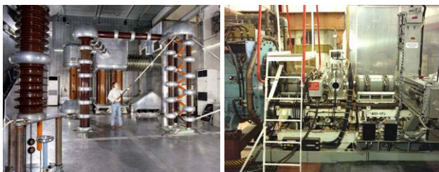
Figure 1: Left, Cockcroft-Walton accelerator, Right, low energy drift space.
