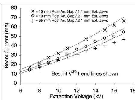
FIG. 4. Beam current vs extraction voltage for different postacceleration gaps and extraction electrode jaw gaps.
