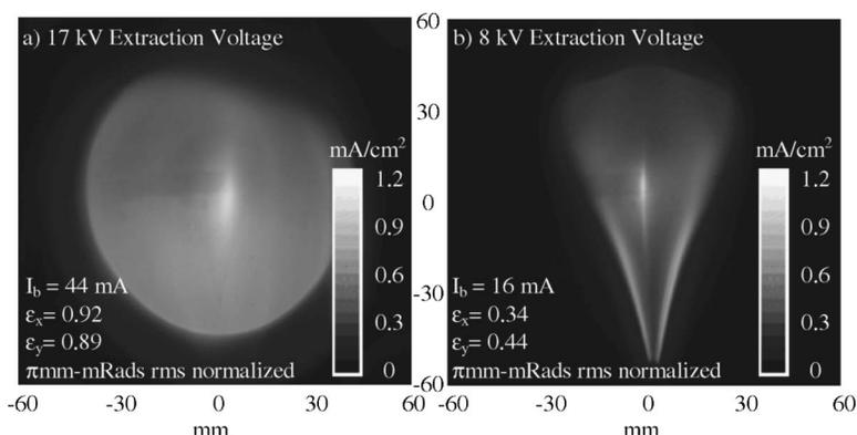
FIG. 2. Beam measurements 615 mm downstream from the ground plane of postacceleration gap with constant postacceleration voltage of 18 kV.
