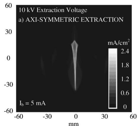
FIG. 5. Beam profile measurement 355 mm downstream from the ground plane of postacceleration gap for axisymmetric extraction.
