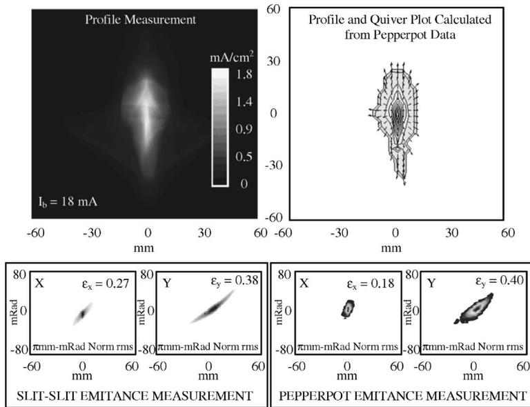
FIG. 3. Beam measurements taken 615 mm downstream from the ground plane of postacceleration gap with extraction voltage=8 kV and postacceleration voltage=18 kV with extraction gap reduced from 55 to 10 mm.
