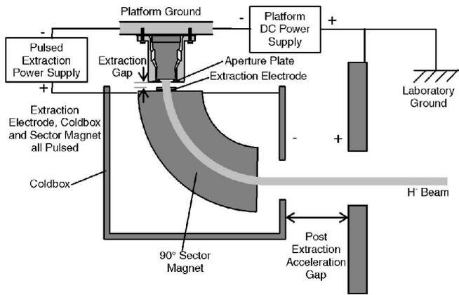
FIG. 1. The ISIS ion source, aperture plate, extraction electrode, sector magnet, and postacceleration gap.
