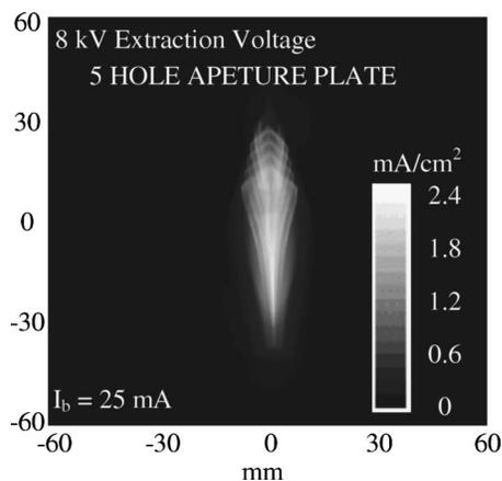
FIG. 6. Beam profile measurement 355 mm downstream from the ground plane of postacceleration gap for a five hole aperture plate.
