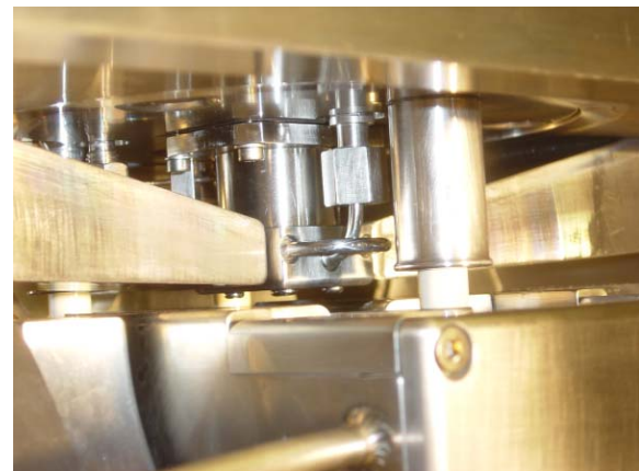
Figure 2: Close-up of the ion source between the Penning pole pieces.
