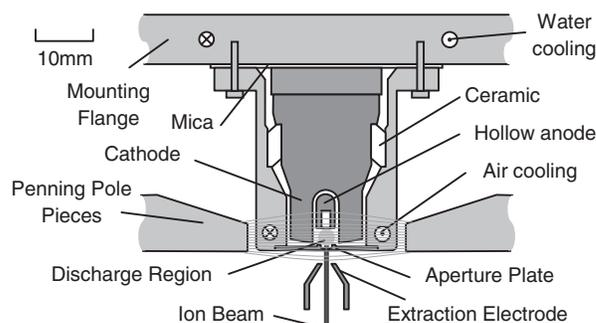
FIG. 1. A schematic of the FETS ion source.
