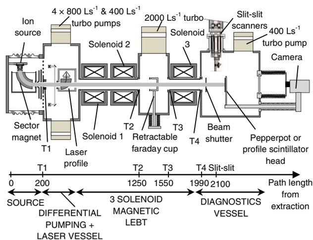
FIG. 2. (Color online) A schematic of the FETS LEBT beam line.
