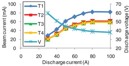
FIG. 5. (Color online) H<sup>-</sup> beam currents and discharge voltage vs discharge current.
