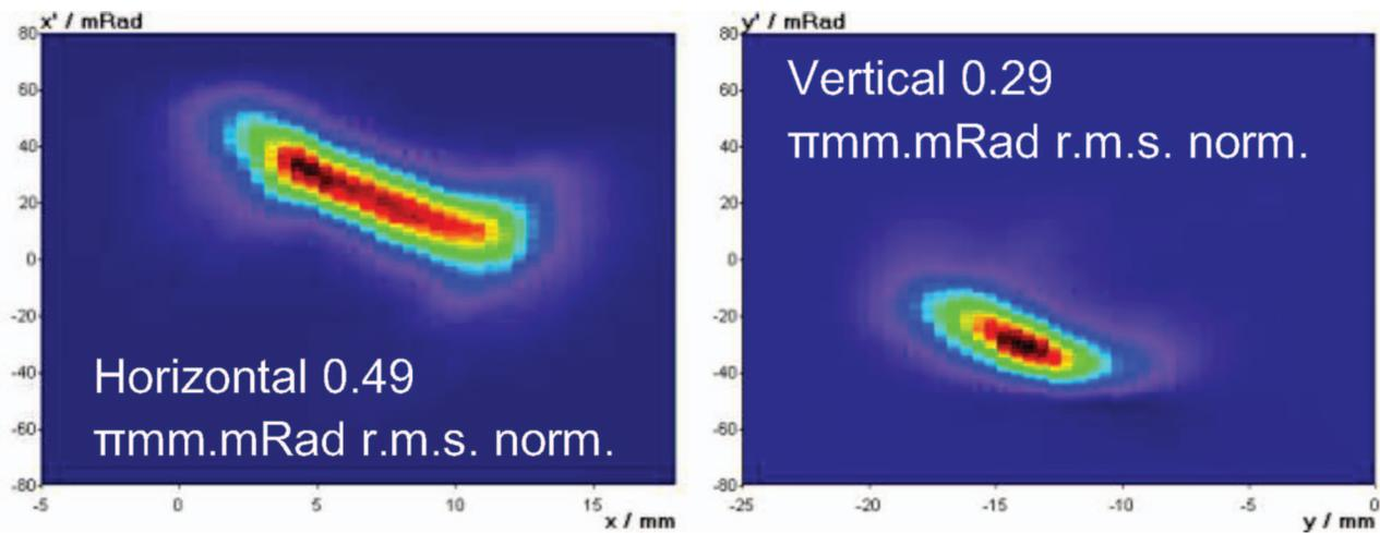
FIG. 10. (Color online) Beam emittance at the entrance of the RFQ for the beam shown in Fig. 8.
