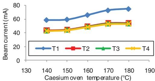
FIG. 7. (Color online) H<sup>-</sup> beam currents vs caesium oven temperature for a 55 A discharge.
