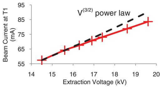
FIG. 3. (Color online) Beam current vs extraction voltage.
