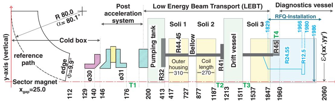
FIG. 1. (Color online) Current set-up of the FETS consisting of a Penning ion source, pumping tank, three solenoids and a diagnostics vessel at the end of the beamline. The LEBT stretches from the post acceleration (PA) through various drift sections and all three solenoids and the diagnostics vessel. The RFQ acceptance is 74 mm in front of the emittance measurement plane at  $z = 1986$  mm. In total, four toroids are installed for beam current measurements and will be referred to as T1...T4.
