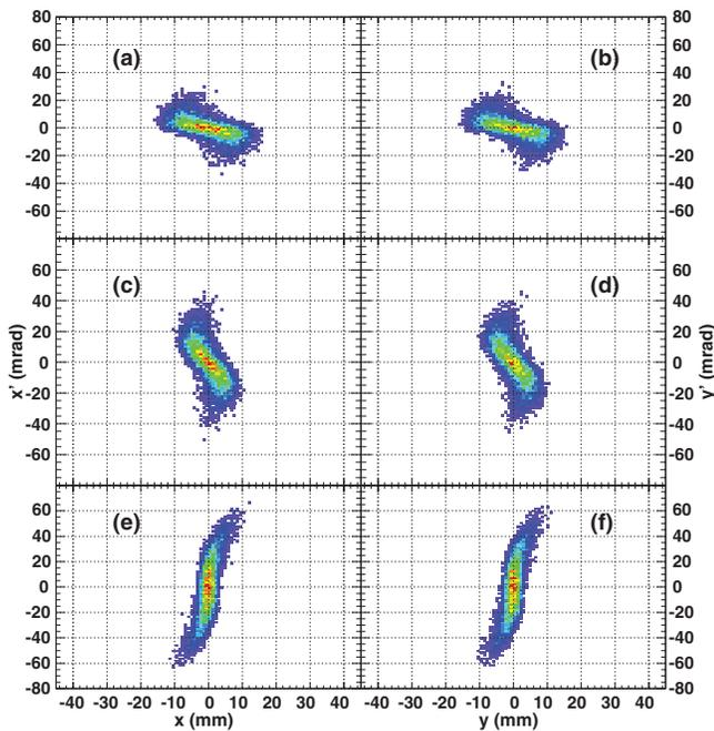
FIG. 6. (Color online) Beam emittance distributions, in  $x$  and  $y$  from GPT simulations. The solenoid current settings are as follows: (137 A, 100 A) for plots a and b; (137 A, 100 A, 150 A) for plots c and d; (137 A, 123 A, 216 A) for plots e and f. The equivalent measurements can be found in Fig. 2.
