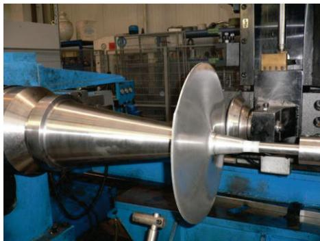
Figure 4: Metal Spinning Process of Beam Stop
